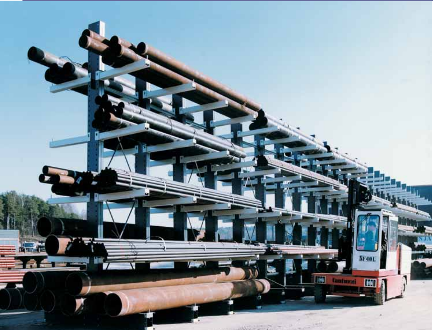
Rack type and dimensions are based on the weight and size of stored goods.
